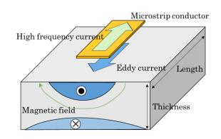
Fig. 6 Schematic diagram of eddy current and magnetic field in a film.
