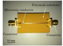
(b) Photograph of the probe **Fig. 1** Schematic diagram and photograph of the probe.
