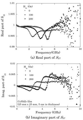
**Fig.** 9  $S_{21}$  of the flexible microstrip-line-type probe (the width of the microstrip conductor was 0.5 mm) when CoNbZr film (25 mm x 25 mm, 5 nm in thickness) was in contact with the probe. Bias fields of 0, 100, and 200 Oe were applied along the easy axis. Ferromagnetic resonance shifted as the bias field increased.
