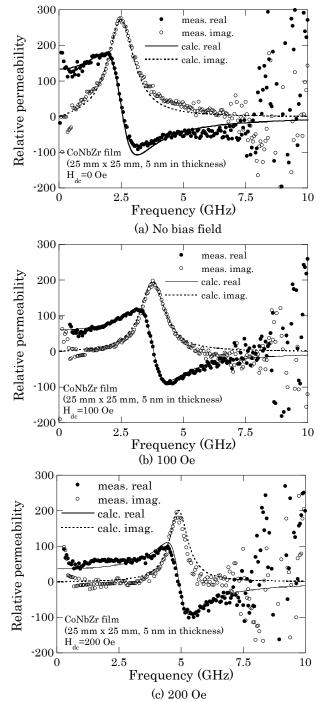
**Fig. 10** Hard axis permeability of CoNbZr film (25 mm x 25 mm, 5 nm in thickness) by using the flexible microstrip-line-type probe. (a) No bias field was applied; (b),(c) bias fields of 100 and 200 Oe were applied to the easy axis.
