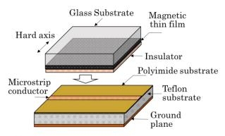
(a) Schematic diagram of probe and magnetic film
