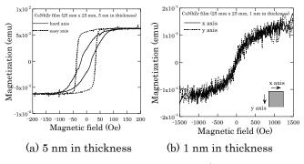
Fig. 7 MH-curve of the CoNbZr film  $(25 \text{ mm} \times 25 \text{ mm}, 5 \text{ nm} \text{ and } 1 \text{ nm} \text{ in thickness}).$
